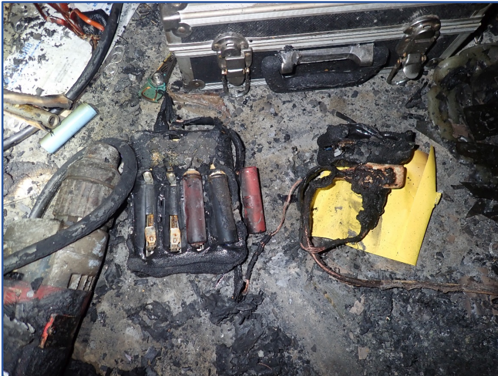
Fig. 3. – Photo of Subject Battery Charger Post Fire
